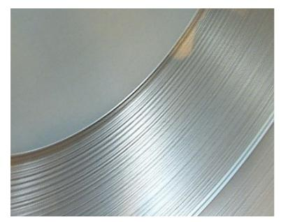
An important indicator of highquality rolling is the even front surface of the coil.
